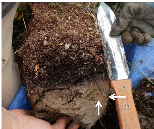
FIGURE A1 Photograph of a soil sample from the closed footslope position containing Oi, Oa, and Bg horizons. The white arrows are pointing to oxidized iron concentrations observed within the Bg horizon. Oxidized iron concentrations are observed in the footslope soils under both open and closed cover
